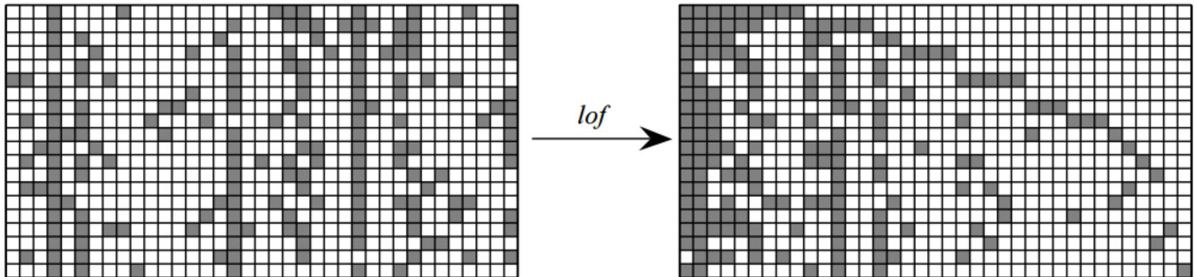
A **many to one** mapping! Order the columns from left to right by the magnitude of the binary numbers expressed by that column, taking the first row as the most significant bit.
